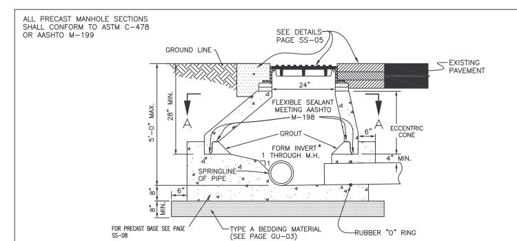
FOR IN LINE MANHOLES THE PIPE MAY BE INSTALLED THROUGH THE MANHOLE BASE AND THE TOP HALF REMOVED.
